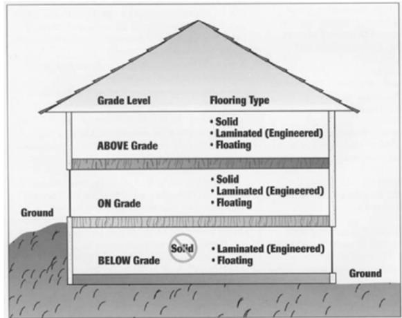
*If any part of the soil surrounding a structure is above the floor of any level, consider that level below-grade. This includes walk-out basements. In addition, the surrounding soil should be sloped away from the structure with at least 6 inches of fall over the first 10 feet.*
